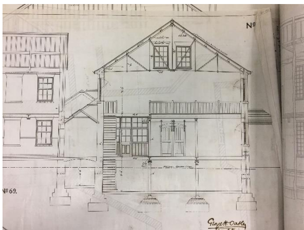
Image 5, section through steel trussed roof construction. (Bristol University, 2019)
