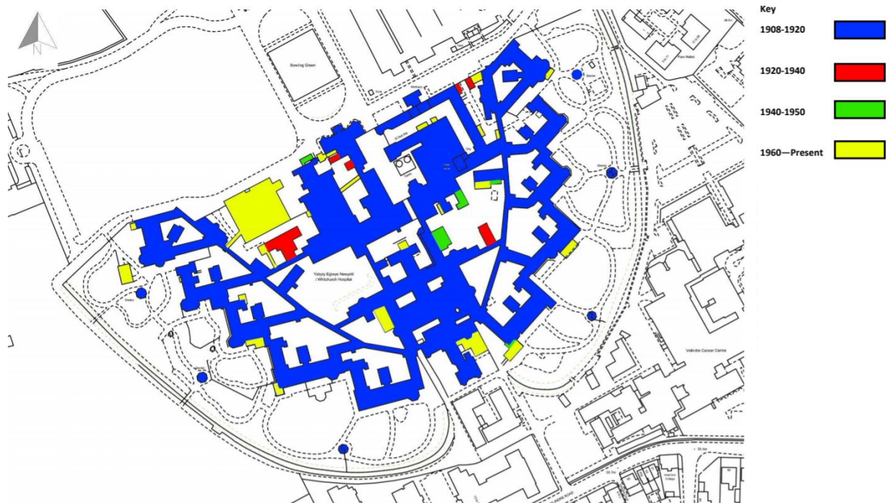
Figure 4: Whitchurch Hospital. Building Morphology of main hospital building 1908 – present (Hayes 2020, p. 4). (Do not scale from drawing)
