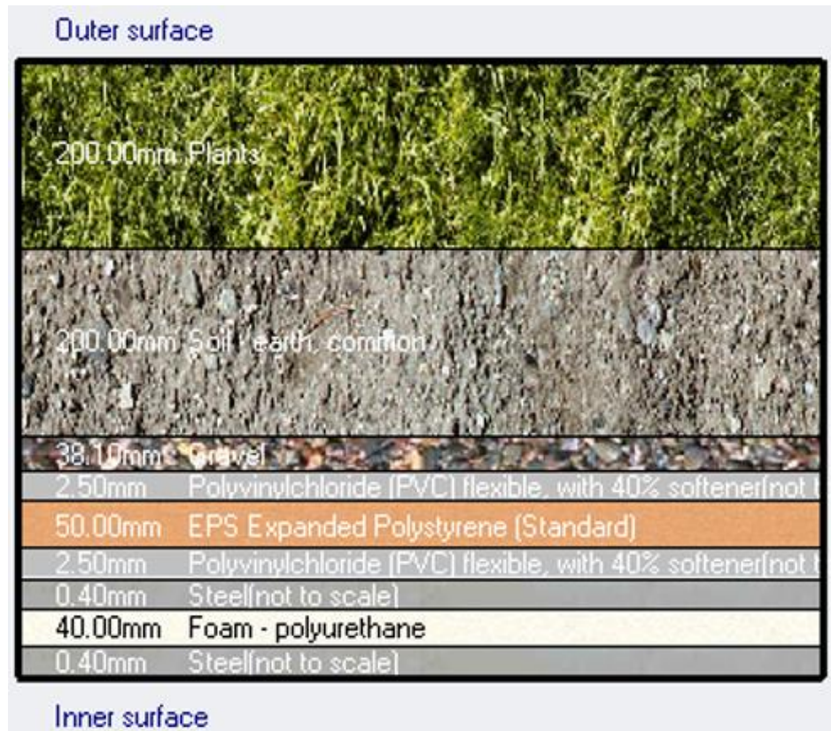
Figure 8 Green Roof Structure Modelled on DesignBuilder
