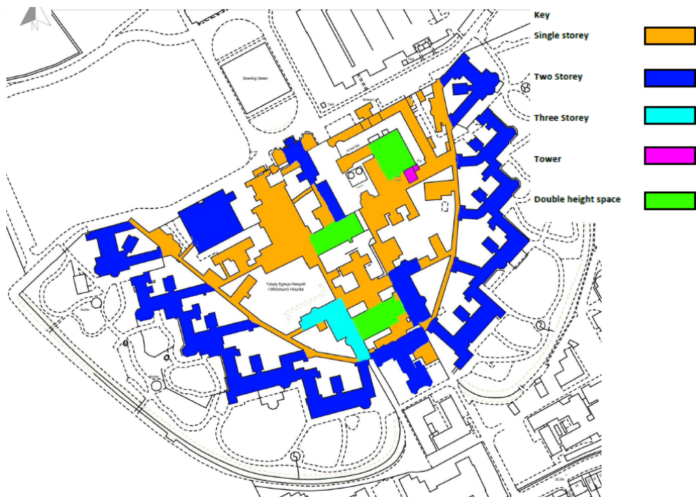
Figure 6: Range of Buildings at Whitchurch Hospital (Hayes, 2020)
