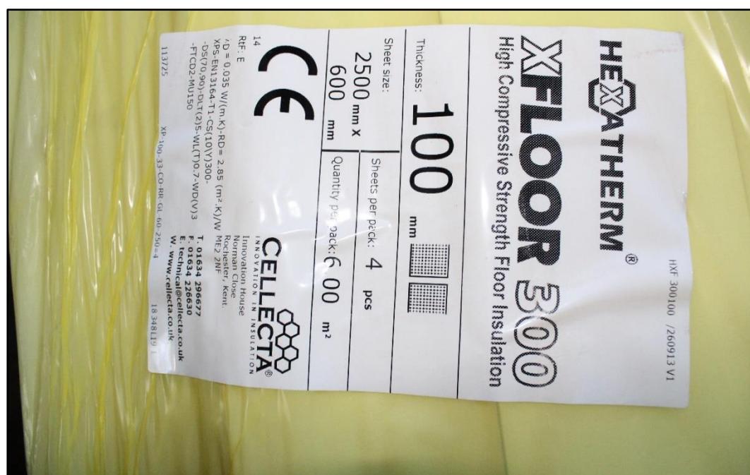
Figure 28: High density polyurethane insulation board information sheet (Source: Gwynne, 2019).
