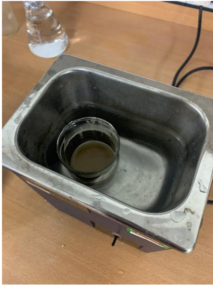
Figure 48 Process of Separation, Aggregate from Binder, Joe Moriarty.
