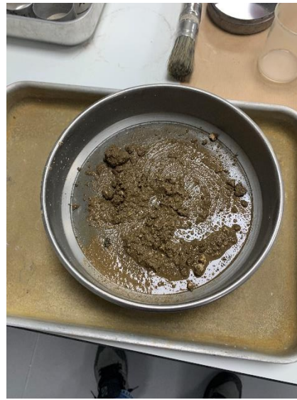
Figure 48 Process of Separation, Aggregate from Binder, Joe Moriarty.
