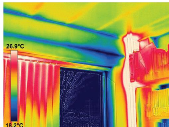
Figure 3.9 – Thermography: identifying thermal bridging (Young 2015)
