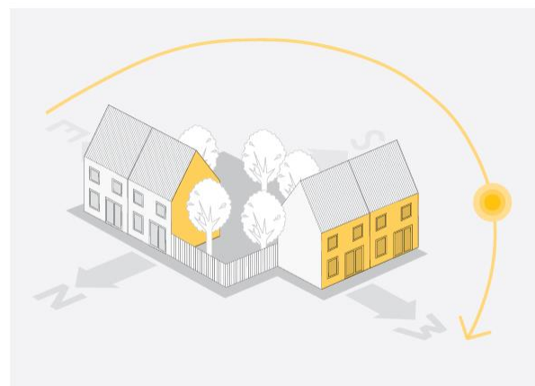
Figure 3.2 – Orientation and solar gain (NHBC Foundation 2012)
