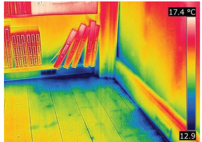
Figure 3.8 – Thermography: identifying air tightness with draughts impacting surface temperatures visible (Young 2015)
