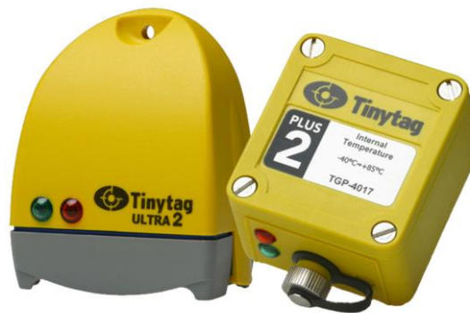
Figure 3.11 – Tinytag data loggers (Gemini Data Loggers [no date])
