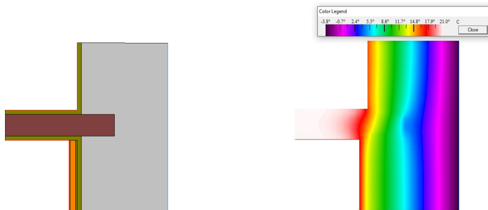
Figure 3.13 – THERM temperature gradient modelling of a solid wall with application of IWI (Author's own 2019)
