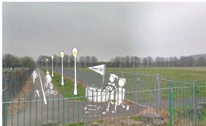
Street lights on long quiet routes and separate cycling from walking to ensure safety
